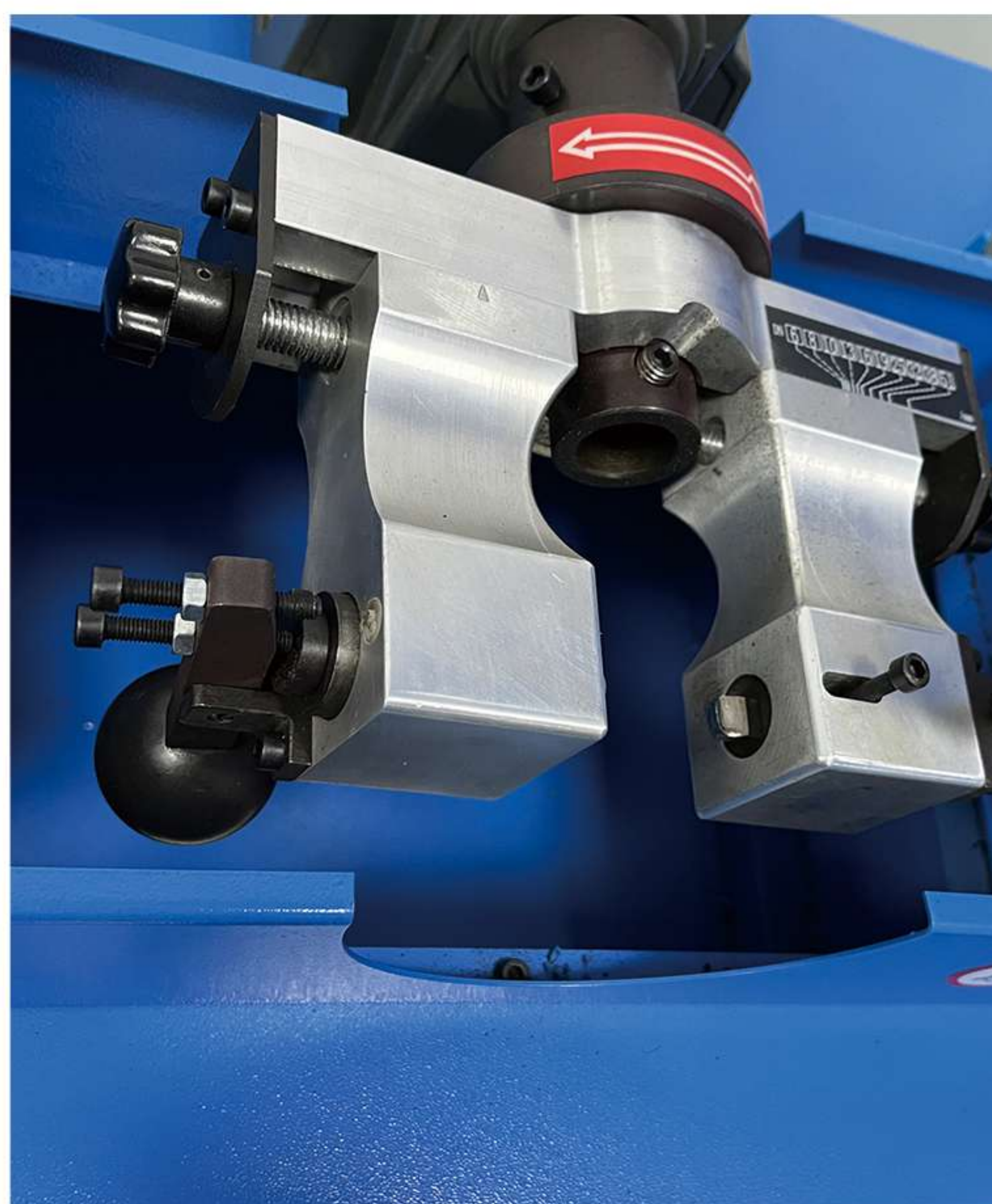
DEVICE FOR PROTECTING STEEL WIRE LAYER
